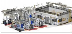
The primary method of scan-to-BIM is to use 3D laser scanners to capture a high-density point cloud of a physical building, structure, or site, which leads to the creation and maintenance of a BIM model that reflects "as-is" conditions.
