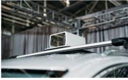
Ex-Apple engineers working for Aeva have developed a solid-state with a range of 200 metres. It's slated to cost "a few hundred bucks" when produced at volume.
