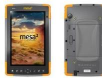
Juniper Systems, Inc. and Industrial Networks recently established a partnership after an extensive, collaborative effort in integrating ATA/AEI long-range UHF RFID tag readers into the Mesa 2 Rugged Tablet. As the only existing solution of its kind, it will serve as a complete identification and tracking system for the railroad industry, as well as other industries requiring long-range UHF RFID tag reading.
