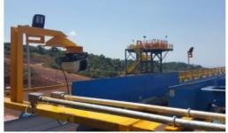
LASE has provided the delivery of 15 LaseBVC conveyor belt measuring systems to the biggest iron ore mining project by Vale in the S11D Complex in North Brazil. In this huge plant the material volume, which is being transported on conveyors needs to be determined by specific measurement applications.
