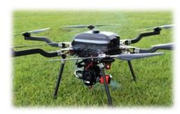
LiDARUSA has announced the integration of their UAV-scanning systems with the Harris Aerial H4/H6 Hybrid multicopters. As surveyors and mappers experience growth, they assume larger and larger projects making longer flight times increasingly important. The Harris Hybrid can provide such flights with lidar and industrial-grade cameras allowing for far greater coverage in a single flight.
