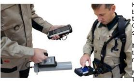
Handheld's Nautiz X8 ultra-rugged PDA has paired with the AT6101C backpack-style mobile spectrometer from Belarus-based ATOMTEX to aid in the detection of radiation. The AT6101C interacts with the Nautiz X8's GPS, GPRS, Wi-Fi and BT functionalities to capture and geo-reference data, then stores the data directly on the mobile unit.
