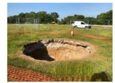
A laser scan has revealed a huge underground void after a sinkhole appeared in a Buckinghamshire playing field. After the sinkhole appeared in a field in the town of Wooburn Green, the local parish council contacted land surveyors and geospatial engineers, Geoterra, to carry out a 3D laser subsurface scan and video survey.
