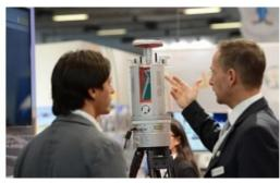
RIEGL have shown off their VZ-2000i terrestrial laser scanner. The device features two on-board processors that enable it to run multiple parallel processes. While scanning in the field, the device can perform registration, geo-referencing, and orientation of data simultaneously, and in real time.
