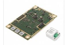
GNSS receiver manufacturer Septentrio has announced the addition of the AsteRx-i S to its GNSS/INS product portfolio. The AsteRx-i S combines Septentrio's compact, multi-frequency multi-constellation GNSS engine with ultralight external industrial-grade MEMS-based IMU. Calibrated for wide temperature ranges, the AsteRx-i S delivers accurate and reliable GNSS/IMU integrated positioning to the centimetre level as well as full attitude at high update rates and low latency.
