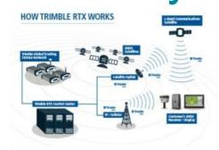
Trimble has announced that its RTX GNSS corrections technology can now achieve horizontal accuracies better than two centimetres, with start-up times also being improved. Users can now achieve full accuracy in less than 15 minutes, and as fast as one minute in select areas where RTX Fast network infrastructure is available.
