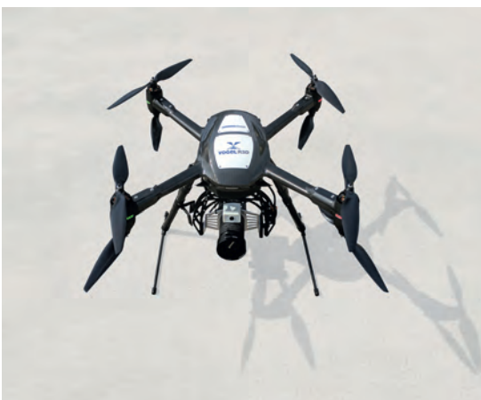
▲ The Vogel R3D system comprises an Aerialtronics drone.
