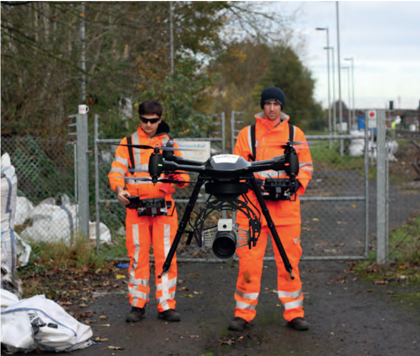
▲ A successful survey was completed with the Vogel R3D at Guildford in Surrey, one of the busiest stretches on the British railway network.
