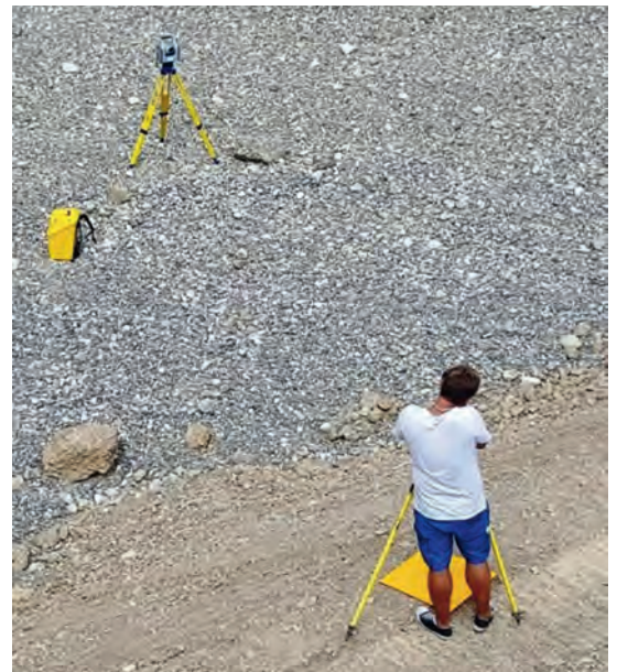
▲ Figure 3: Yellow square used as ground control point from which the Trimble SX10 was orientated.
