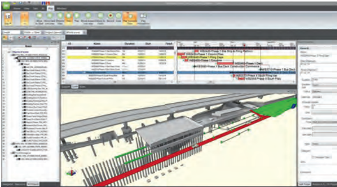
Synchro 4D construction modelling of Crossrail Station.
