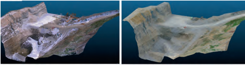
▲ Figure 4: Digital surface models generated from TLS (left) and RTK-only UAS (100m flying height).
